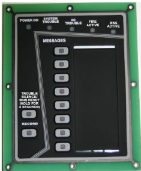
Keypad for Voice Message Selection located inside SP40SD
