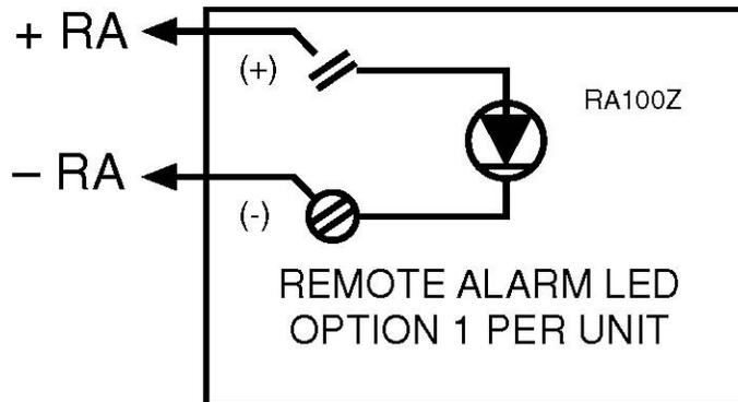
**Wiring for Intelligent Non-Relay Duct Smoke Detector: continued**
